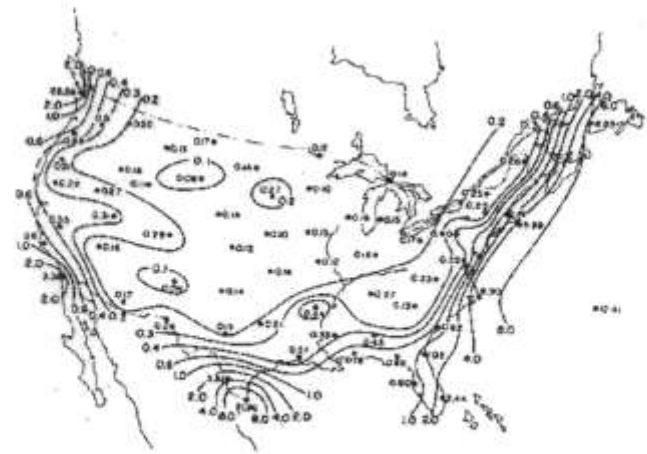
Penetration of seaspray inland in the USA Ocean derived Chloride ion concentration from Junge 1961
